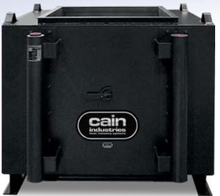
Boiler: 500 HP Steam Boiler Exhaust gas temp *before* economizer: 430° F Exhaust gas temp *after* economizer: 305° F BTU transferred into boiler feedwater: 631 MBTU/hr Total cost installed: \$23,280
