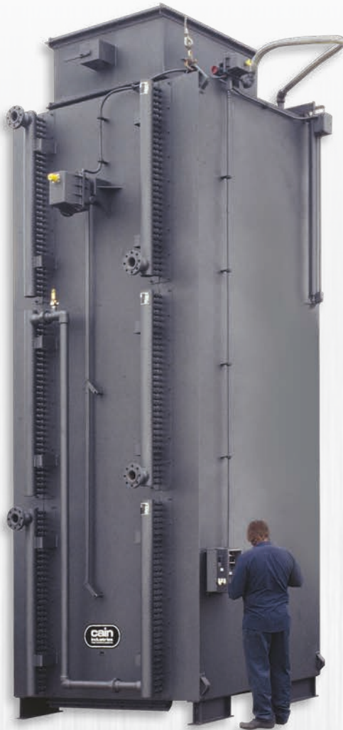
Vertical flow RTR shown with optional timed automatic sootblower assemblies. This unit uses three sets of traveling carriages with high velocity cleaning nozzles.
